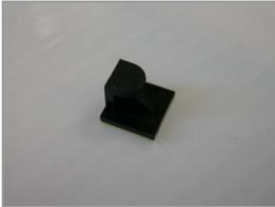
The spacer support is good for fixing ECM-S48XX in 20mm width, ie dim. 76(L)x20(W)mm or 305(L)x20(W)mm, to where one would like to use. Constructed of NYLON 66 (UL) material, the spacer support is designed to use for indoor environment, rated Flame Class 94V-2. Color BLACK.
